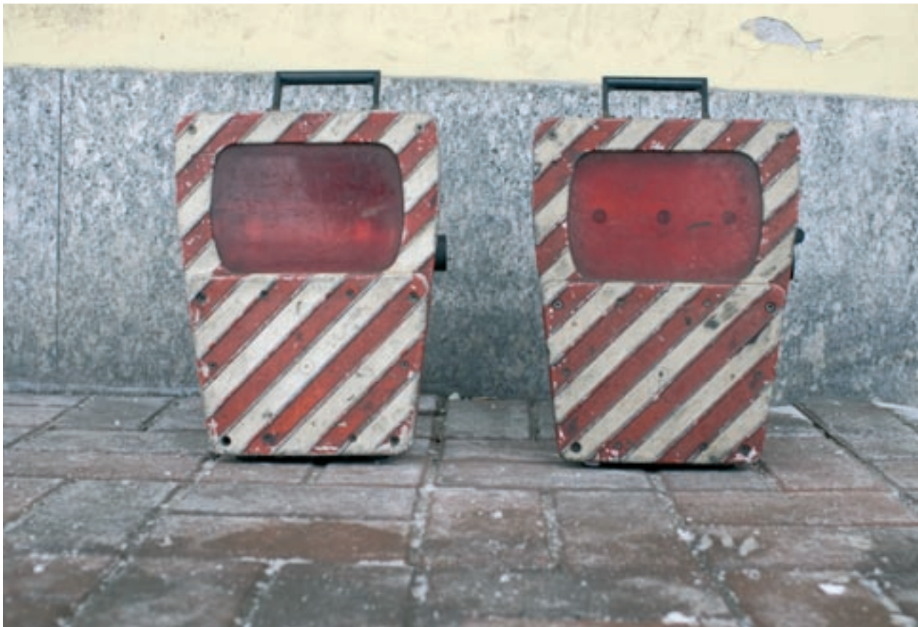
Photo 9 – Tail lights required for operation in Italy awaiting attachment at Brennersee station
