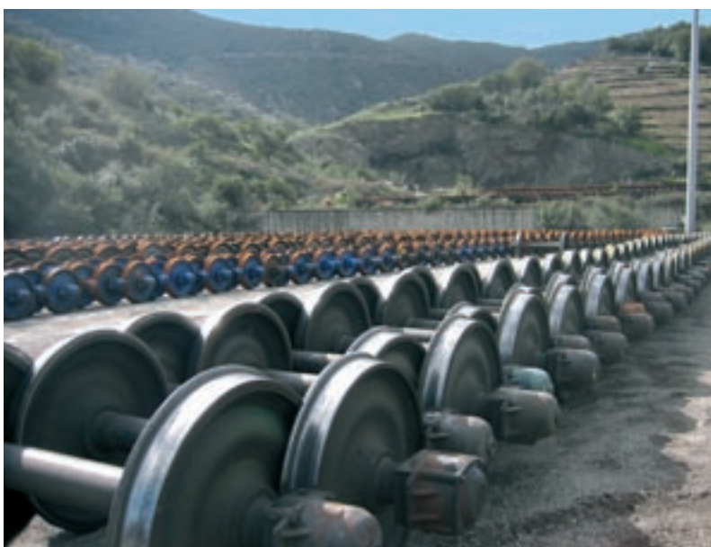
Photo 6 – Stock of wagon axles at the TRANSFESA gauge changing facility at Cerbère on the France / Spain border
